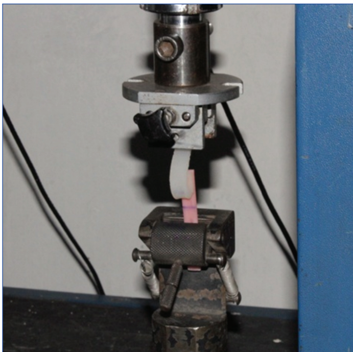
[Table/Fig-4]: Prepared acrylic and silicone specimen placed in the universal testing machine for the peel bond test.
